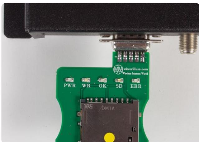
The update process is now complete. Turn off the controller and remove the SD programmer. The control unit can now be put into operation again as usual.
