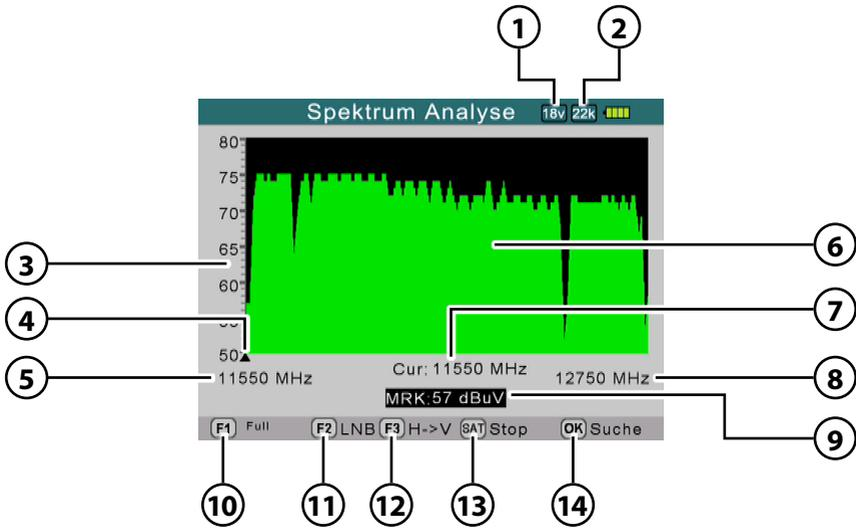
1. Displays the current voltage of the LNB. The values are: 13 V, 18 V or OFF.
