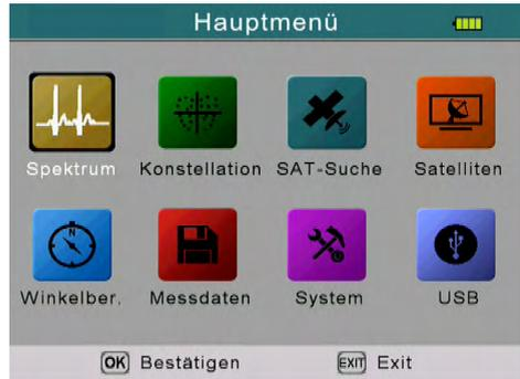
Use the ▲▼ or ◀▶ buttons to navigate the menu. Press OK to enter the submenu. With MENU return to the main menu.
