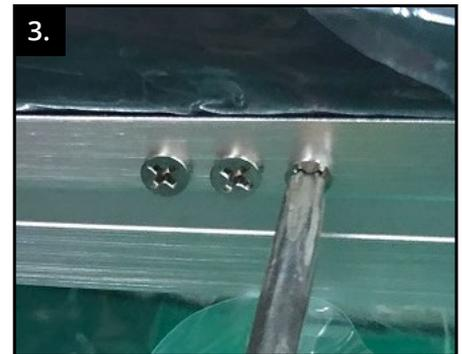
3. Unscrew all phillips screws (12 pcs.) from the bottom of the display.
