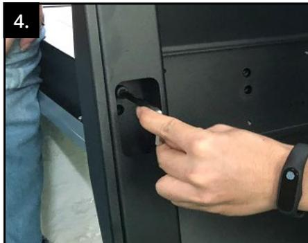
4. Attach the stand and fasten it with the 10 allen screws.
