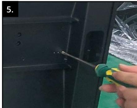
5. Additionally secure the stand with the 12 phillips screws.
