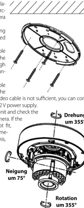
8. After you have determined the correct position, you can unscrew the glass dome housing again. Press firmly on the camera base and fix it by turning it clockwise.
