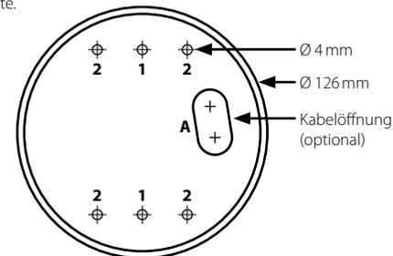
**Note:** The hole of the cable hole is required only when the outlet is used to lay the cable.
