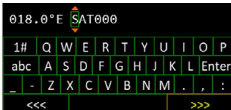
2. Press the **F2 key** to add a satellite. A keypad is displayed where you can enter the name and the degree.
