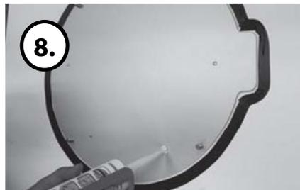
Re-apply glue to cover bolts assembled
