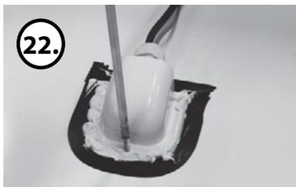
Fix cable holder on the car roof with 3 of M4x20.
