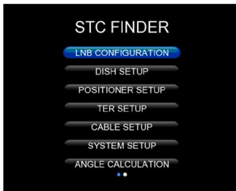
Use the ▼▲ keys to move the cursor up or down in the menu. Use OK key to confirm a selection. To escape the menu system at anytime, press EXIT key.
