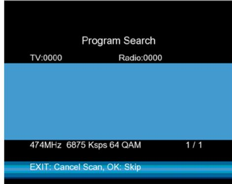
**3. Auto Scan:** Scan all range of frequency and bandwidth. It costs time to do Auto Scan, user can press.
