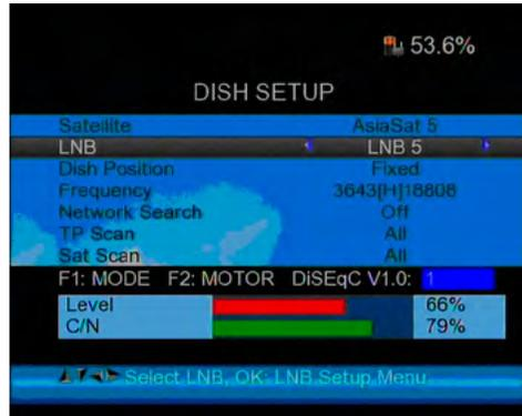
**1. Satellite:** Press OK button to display the satellite list. Select the satellite you want to check with pressing ◀▶ button. You can also press ▼▲ to select the satellite. Press <OK> to confirm your selection.
