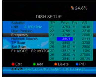
**Add:** Press GREEN (H/V) button to add Frequency using the numeric keys. Press ▼▲ key to select "Pol". Press OK button to confirm the operation and save the result.
